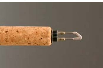
RT-A (1/4") Round Tip. This tip is the largest of the rounded tips an is used for concaved areas, such as under the neck and where the leg joins the body. This tip style will follow concaved surfaces without digging into the wood.
