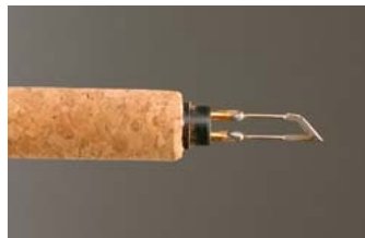
Replaceable Tip-Bob Guge. Used for outlining feathers.
